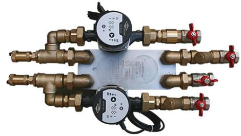
*The set is comprised of:* a plate exchanger with the appropriate number of plates (selected depending on the power of the fireplace insert), two circulation pumps, two filters, two deaeration valves, a check valve (on the central heating system), stop ball valves. Additionally, the set also includes brass fittings for connecting particular elements.
