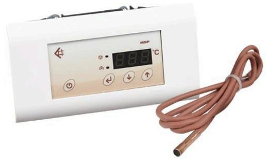
Apart from its basic functions, the controller also informs about the fact that the alarm temperature has been exceeded, protects the installation against freezing by automatically switching off the central heating pump if the temperature measured falls below 4°C and against self-activated switching from the stand-by mode after detecting an increase in the temperature of the liquid in the installation.
