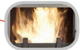
**large combustion chamber** - lined with Acumotte (system of holes in the back wall is in charge of the aeration of the combustion chamber)
